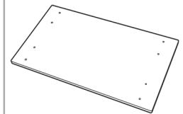
After tightening the screws, use a drill to make mounting holes on the backside of the tabletop through the 8 mounting holes on the side brackets.
