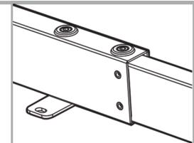
Loosen the hex head screws that fix the adjustable junction, but don't completely take out the screws.
